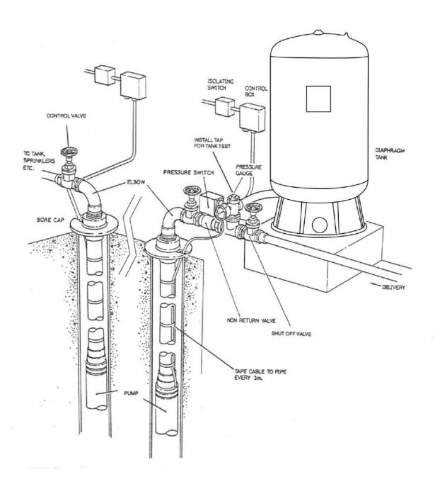
Pump connected for manual operation
